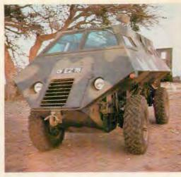
Above: Front view of Bullet, prototype armored infantry fighting vehicle, built by Rhodesian Armored Corps. After 10,000-kilometer road test, Bullet will be blown up by captured Russian landmine to determine its resistance to blast and heat.
